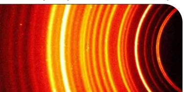
suitable for high-throughput and fast PXRD measurements. In addition, very small quantity of material is needed to perform 2D-PXRD analysis using modern instruments.
